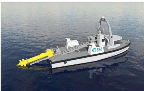
*AUV or Towed Sonar configuration*
