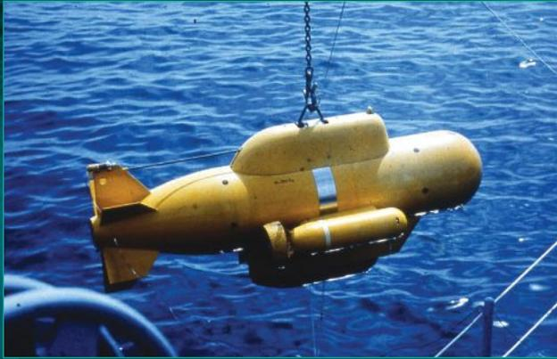
• The *Poisson Auto-Propulse* (self-propelled fish) or PAP was developed by ECA in the 1970s for underwater mine detection. It had to operate silently, because the slightest noise could trigger a detonation. Sounds dangerous, but the first PAP is still in service for the French Navy, forty years after deliver. Photo courtesy of ECA.
