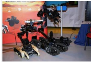
The family of ground robots presented by the ECA Group, left to right a Cameleon, an Iguana and a Cobra Mk2. © P. Valpolini
