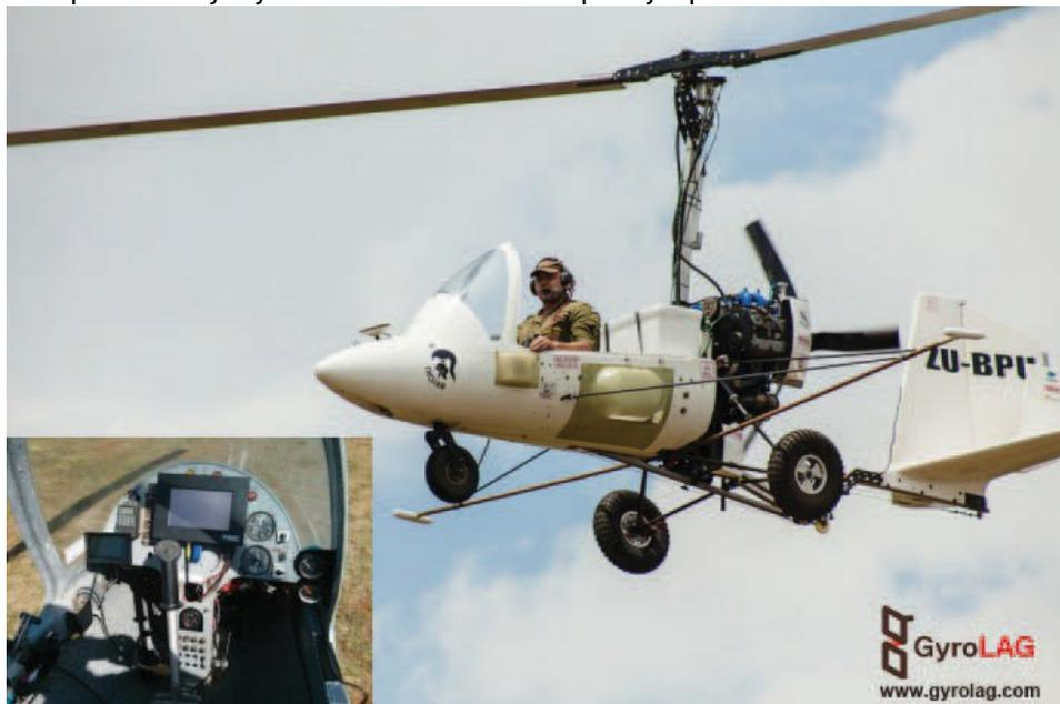
FIG 1 – GyroLAG South African gyroplane Trojan type with GyroLAG's FLAME (fluxgate airborne magnetics) gradient magnetic system. Inset: cockpit view with navigation computer (centre) and data acquisition pilot display (left).
