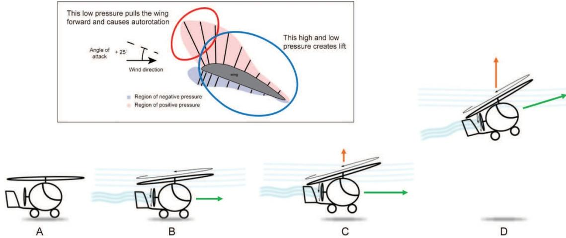
FIG 2 – Flying principles of a gyrocopter. (A) Standing still; (B) propeller generates forward motion (green arrow) and air flows over the rotor blade; (C) rotation generates lift (orange arrow) - see insert; (D) lift overcomes gravity. Insert - schematic of pressure distribution around a wing.
