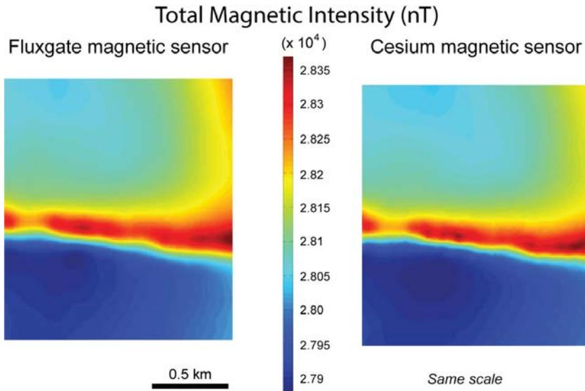
FIG 4 – GyroLAG fluxgate on-board a gyrocopter (left) versus traditional Cesium airborne magnetic mapping on-board a fixed-wing aircraft (right; data from South Africa Council of Geosciences).
