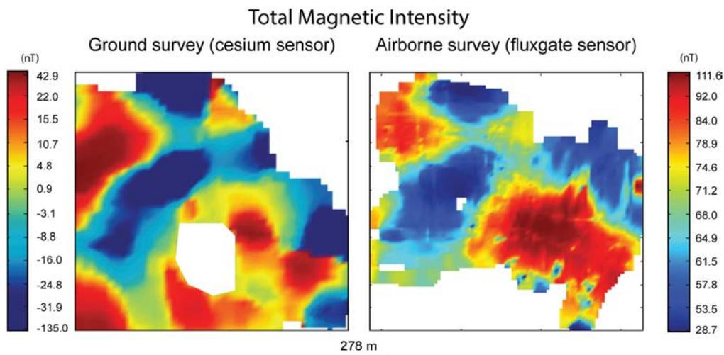
FIG 5 – Airborne fluxgate magnetic mapping (right) versus Cesium ground magnetic mapping (left) (after Bouiflane, 2008). Both maps cover the same area but the effective surface surveyed varied slightly.
