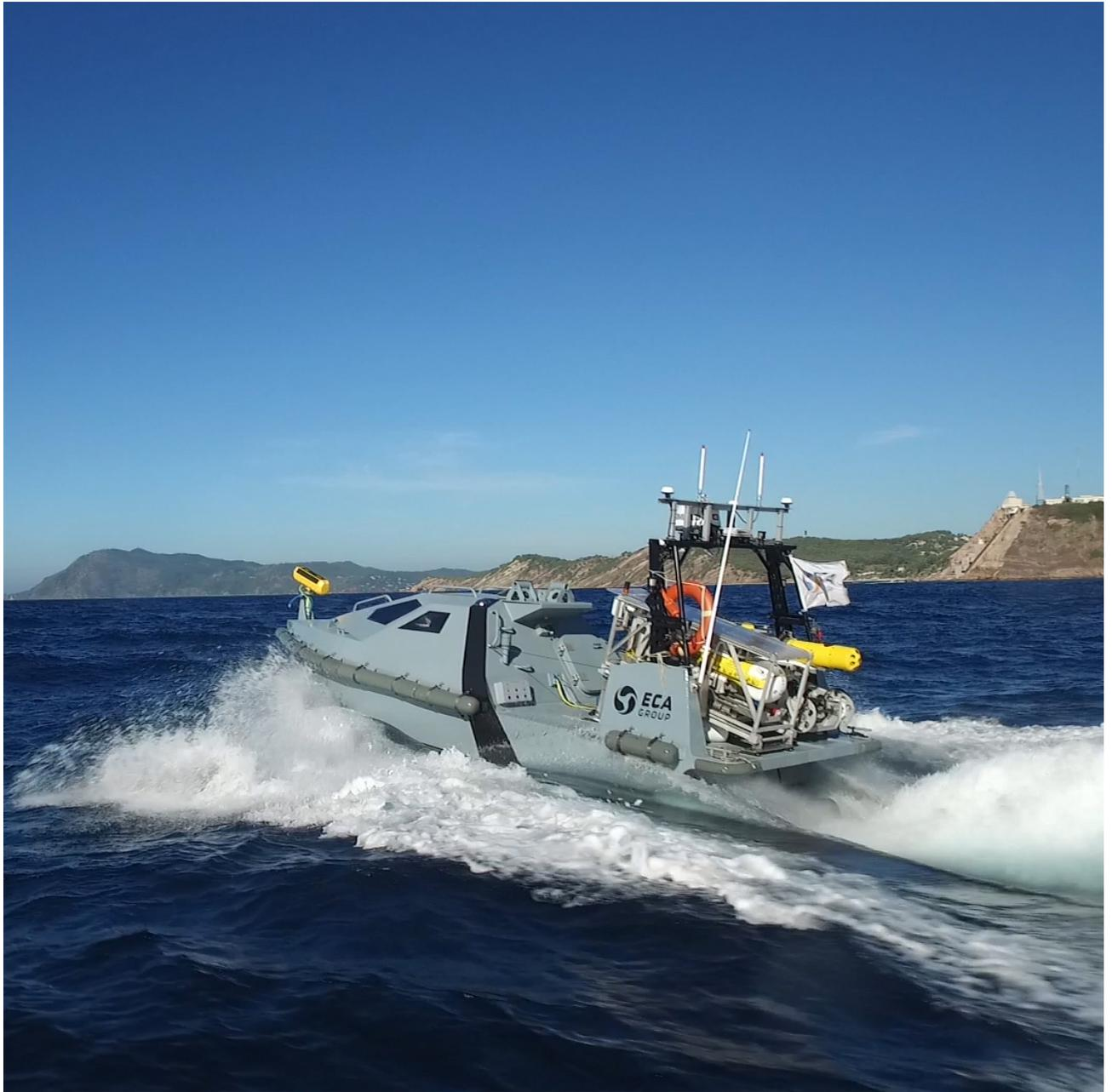
*Illustration of a drone system based on Unmanned Surface Vehicle USV [INSPECTOR MK2](#) which can autonomously deploy underwater robots [SEASCAN MK2](#) (inspection robot) and [K-STER C](#) (minekiller underwater robot).*
