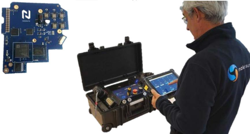
SmartCo is a solution that uses reflectometry, a diagnostics method based on the principle used by radar. The innovation behind the SmartCo solution is that it combines reflectometry with communication using the new Orthogonal Multi-tone Time Domain Reflectometry (OMTDR) method. This OMTDR technology is able to perform preventive maintenance and detect faults within a wired network more quickly.
