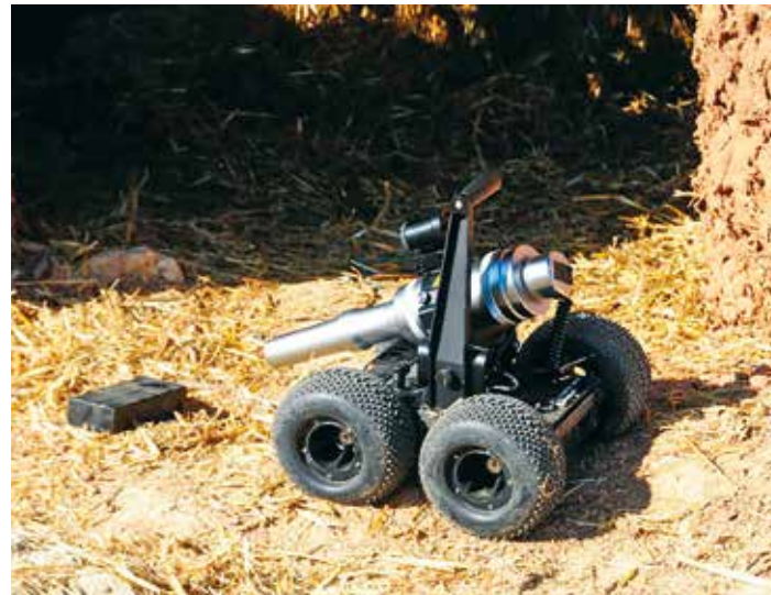
UGV COBRA MK2 E equipped with a Tilttable Disrupter Support
