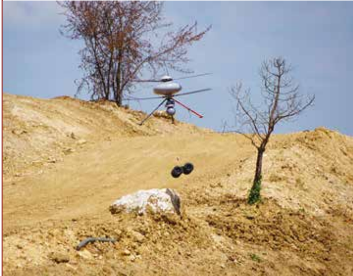
Airborne transportation of UGV COBRA with UAV IT180
