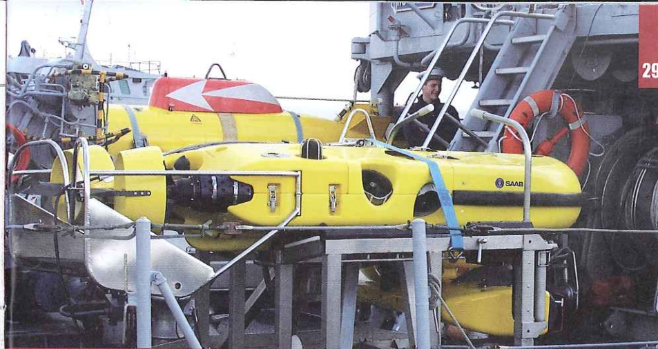
Saab's Double Eagle SAROV can operate either with or without a tether at depths of 500m and speeds of 8kt. (Photo: author)
