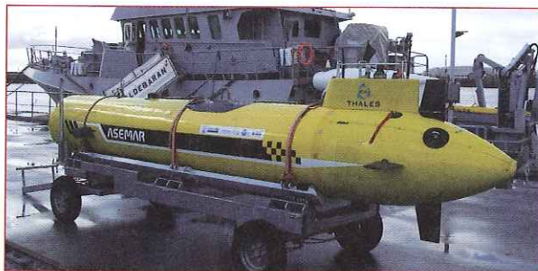
Thales is involved with the development of the Asemar AUV, which is equipped with a side-scan synthetic aperture array sonar, and is designed for MCM work and hydrography. (Photo: author)
