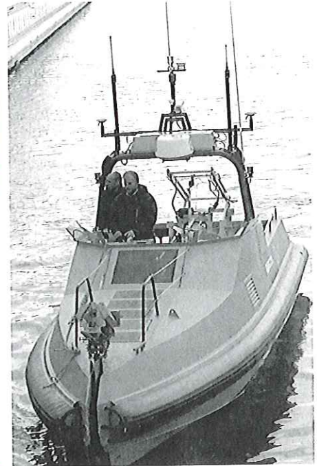
Fig. 3: ECA presented on the River Seine their Unmanned Surface Vehicle INSPECTOR on the river Seine with its forward looking sonar for minehunting, intelligence surveillance and reconnaissance, maritime interdiction operations and coastal/port security (here lifted out of the water). The USV was operated from the bateau mouche (where the selected guests were embarked), although for Seine river legislative reasons two operators had to be onboard the USV, and results of the sonar scan were transmitted to a screen onboard the Seine boat. (Photo: wl / Mönch Publishing Group)
