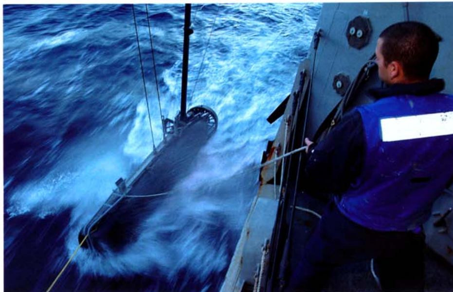
Lockheed Martin's AN/WLD-1(V) remote minehunting system was deployed by the DDG-51 Flight IIA destroyer USS Bainbridge in December 2007 in an exercise off the Spanish coast.
