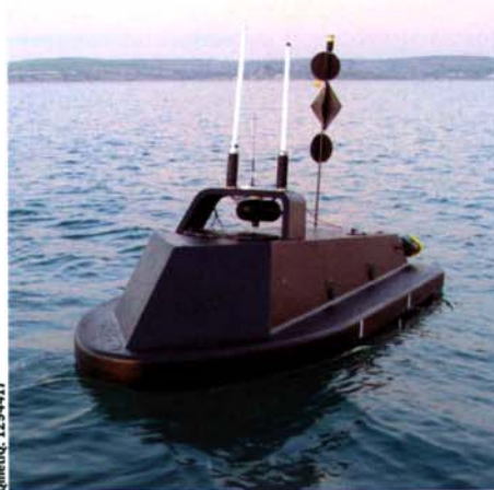
(Above) QinetiQ's Sentry is a fast, low radar-cross-section unmanned reconnaissance and surveillance craft that marries military design requirements with a compact jet ski-type vehicle based on a high-speed planing hull.
