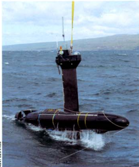
ASV's SASS 6M Mk II vehicle was trialed in June 2007 as part of the UK's USV CCD programme.
